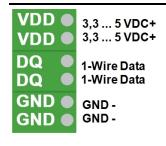
One of the terminal points VDD/DQ/GND is required for the connection of a sensor. The additional three clamping points are for
